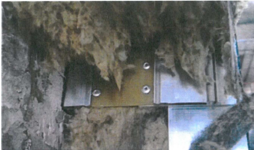
Fig. 5. A passive bracket after tests carried out for the purpose of the opinion [17].
