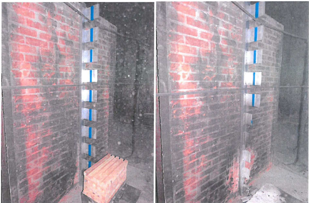
Fig. 7. A general view of the sample during and after testing, according to PN-B-02867:2013-06 - KW4 PAS brackets
