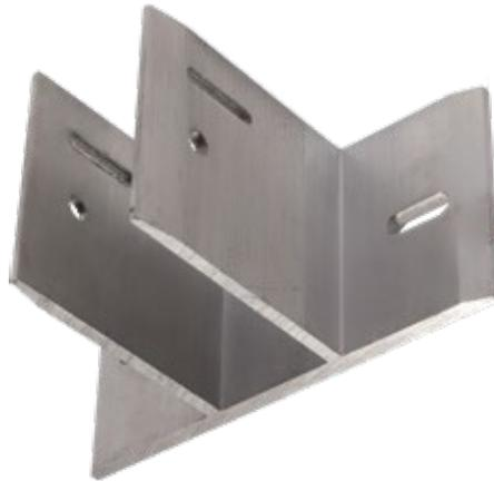
The K1 brackets are a standard solution designed to fix mullions of the façade. The bracket that looks like the  $\pi$  letter provide good access to all dowel bars and bolts as well as the adjusting element.
