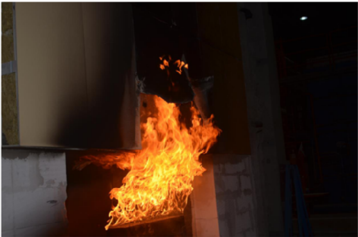
Fig. 6. Picture of the sample element in 7 th minute of the test (workpiece)
